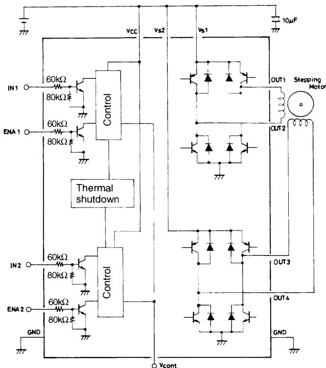
Note: As long as the voltages applied to  $V_{CC}$ ,  $V_{S1}$ ,  $V_{S2}$ ,  $ENA1$ ,  $ENA2$ ,  $IN1$ , and  $IN2$  are within the limits set by the absolute maximum ratings, there are no restrictions on the relationship of each voltage level in comparison with the others (regarding which is higher or lower). (ex.  $V_{CC} = 3\text{ V}$ ,  $V_{S1, 2} = 2\text{ V}$ ,  $ENA = IN = 5\text{ V}$ )
