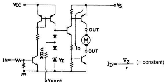
As shown in the above diagram, the  $V_{cont}$  pin outputs the voltage of the band gap Zener  $V_Z + V_F$  ( $= 1.93\text{ V}$ ). In normal use, this pin is left open.
